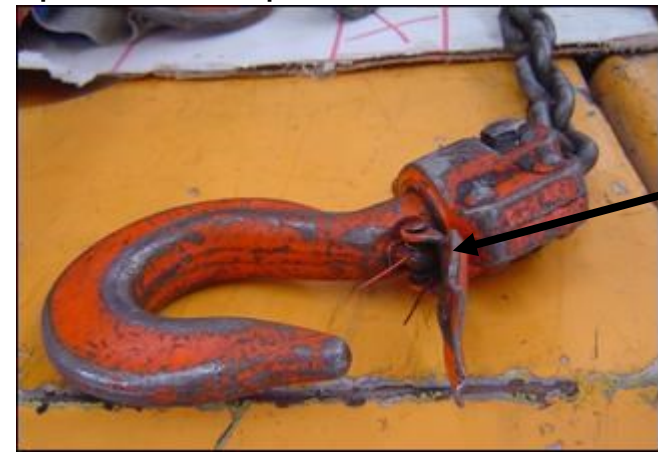
Safety lock damage
